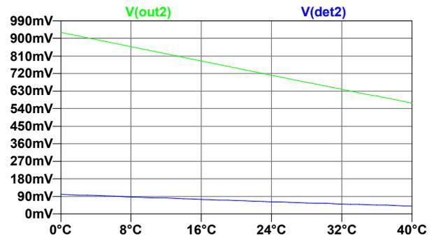
Figure 7. Effect of temperature on log amplifier
