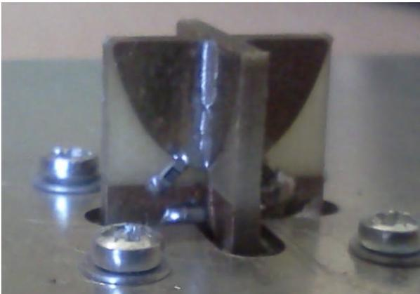
Figure 17. Close up of quad blade antenna
