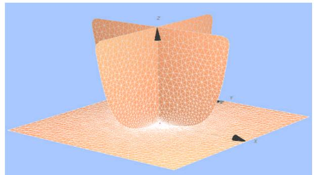
Figure 10. 8mm Quad-blade antenna with increased capacitance
