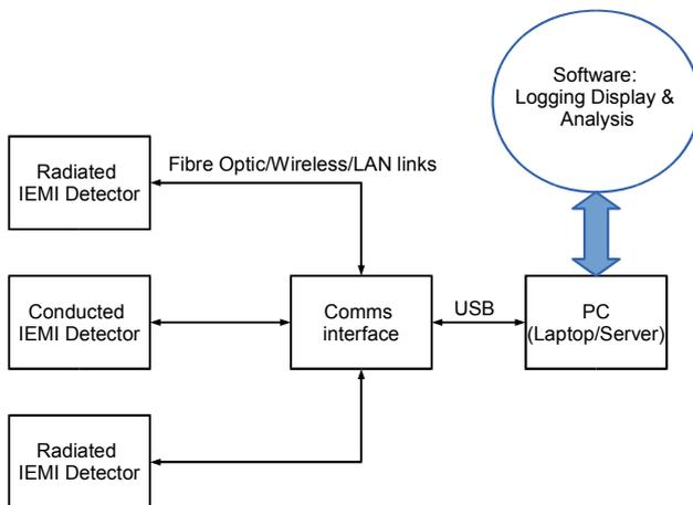
Figure 1. Low cost IEMI detector system concept
