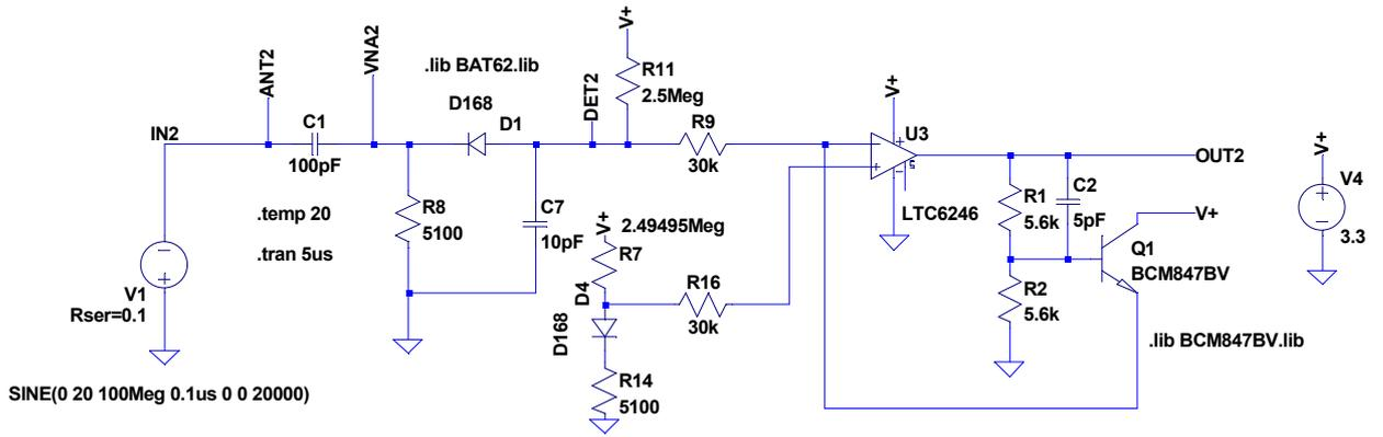
Figure 4. Log amplifier and detector initial design
