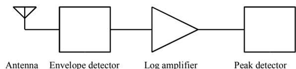
Figure 3. Log amplifier and detector design concept
