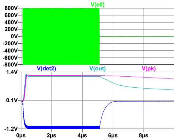
Figure 13. SPICE model of Detector showing time response of the detector to a 100 MHz sinusoidal input. The top trace shows the incident field in V/m and the bottom trace shows the microwave detector output (dark blue), the differential amplifier output (light blue) and the peak detector output (magenta).
