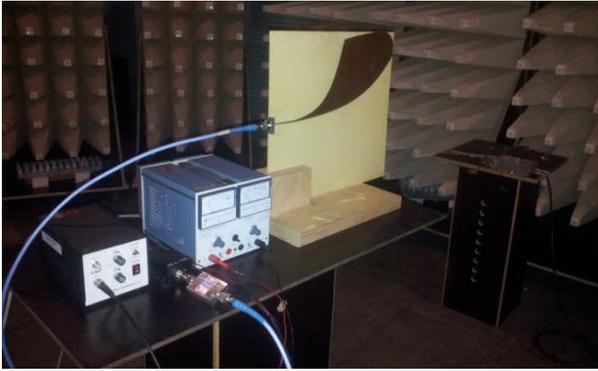
Figure 15. IEMI detector test setup with pulse generator at Rheinmetal's a nechoic chamber
