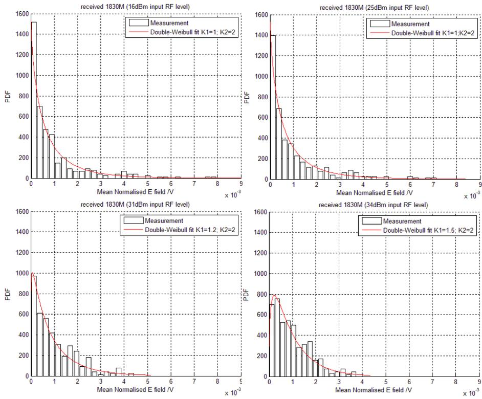
Fig.7 Probability density of mean normalised spectrum of inter-modulation between 2<sup>nd</sup> harmonic and digital clock
