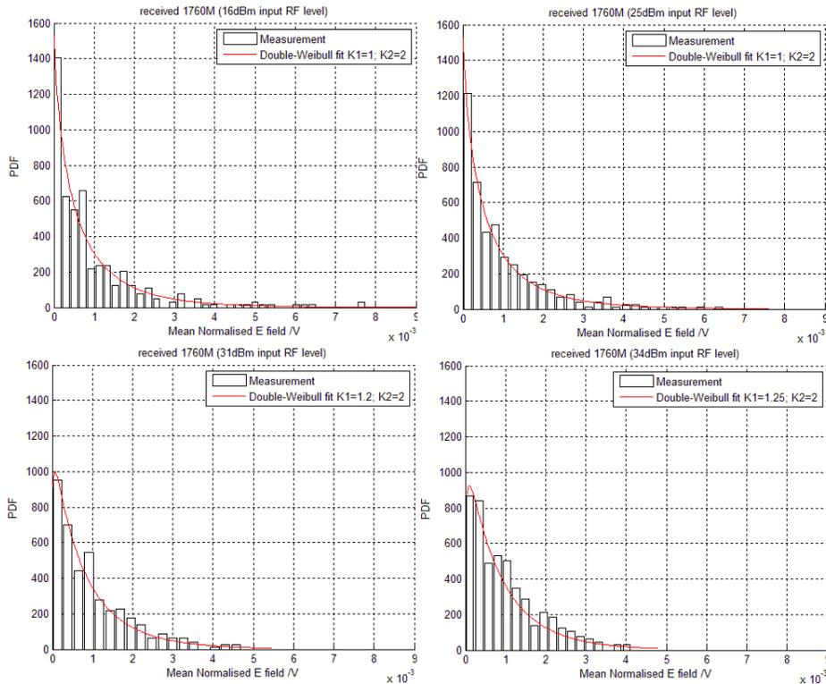
Fig.6 Probability density of mean normalised spectrum of 2<sup>nd</sup> harmonic
