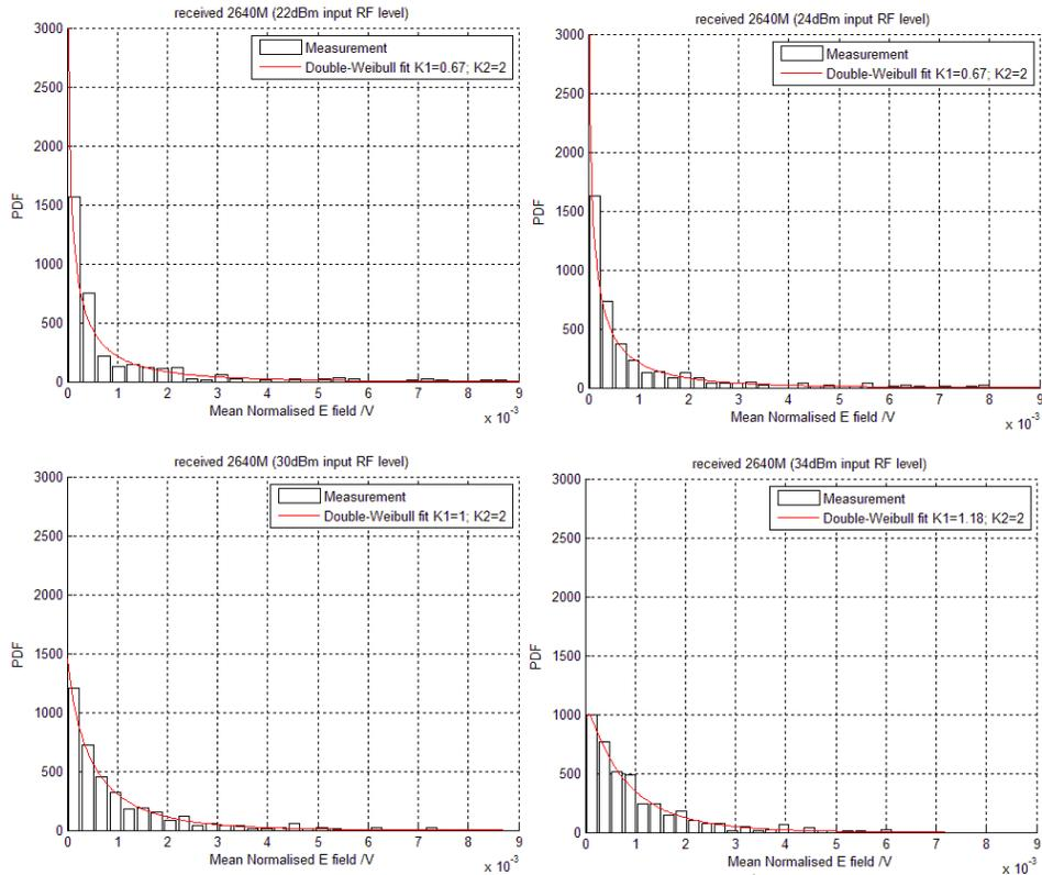
Fig.8 Probability density of mean normalised spectrum of 3<sup>rd</sup> harmonic
