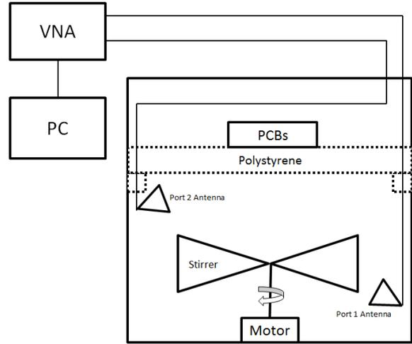
Fig. 3. Side view of the ACS measurement setup.
