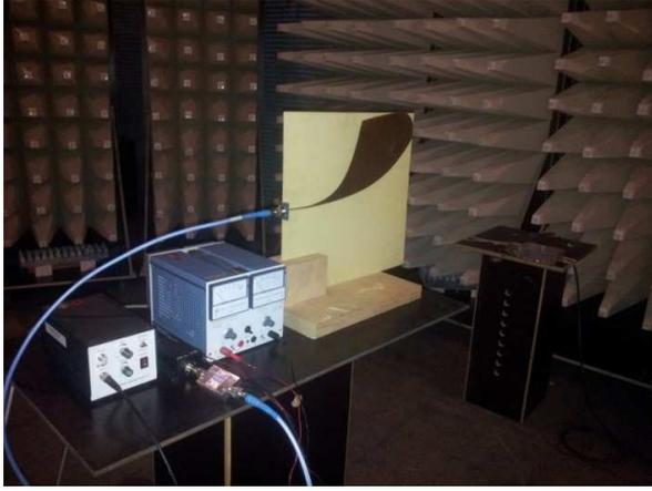
Fig. 4. The low cost IEMI detector prototype under test with double exponential pulse generator at Rheinmetall test facility Unterleuss.
