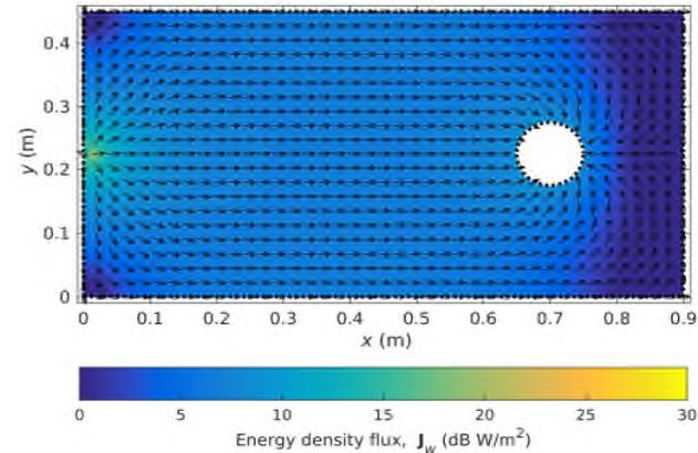
**Figure 4.** Diffuse energy density flux,  $J_w(x, y, h/2)$ , in the cuboid enclosure with an absorbing cylinder with  $\alpha_c^a = 1.0$ .
