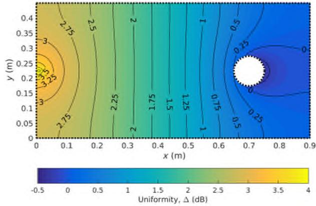
**Figure 3.** The diffuse energy density uniformity for enclosure with absorbing cylinder.
