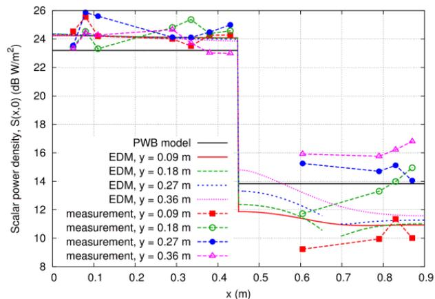
**Figure 8.** Comparing the PWB, diffusion and measured results along different lines in the  $z = h$  plane of the enclosure with partition and absorbing cylinder at 8.5 GHz.
