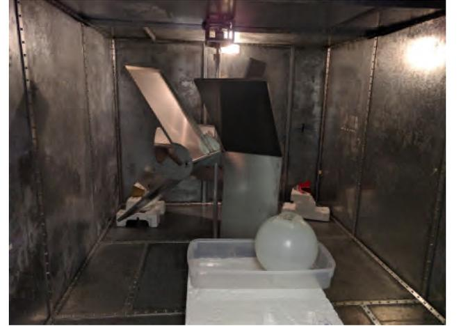
**Figure 4.** Reverberation chamber containing paddle and broadband antennas, loaded with spherical phantom of known ACS.
