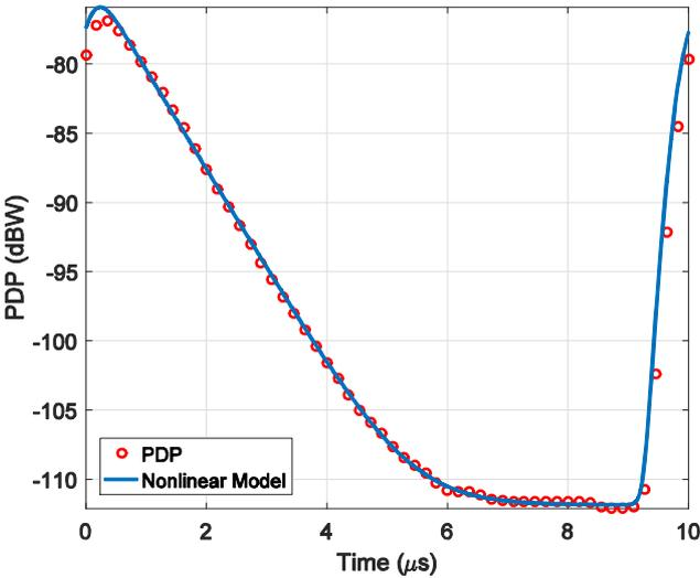
**Figure 2.** Output of nonlinear model fitted to measured PDP at 10GHz (filtered by a 5MHz smoothed cosine window), showing good agreement with the linear part (0-6  $\mu\text{s}$ ), the noise floor (6-9  $\mu\text{s}$ ) and the IFFT artefact (9-10  $\mu\text{s}$ ).
