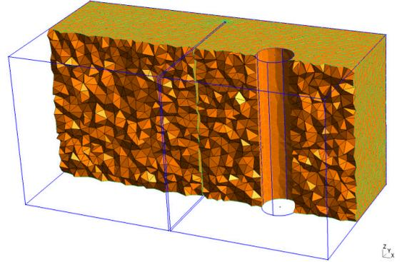
Figure 2: Tetrahedral mesh of the coupled cavities test-case containing the lossy cylinder.
