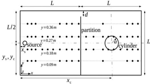
Figure 1: Cross-section of the cuboid cavity used for the canonical examples and validation measurements here and in [4].
