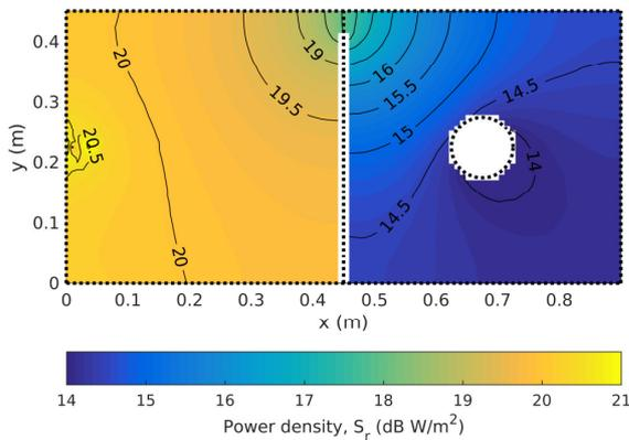
Figure 4: Diffuse power density,  $S_r(\mathbf{r})$ , in the plane at the half-height of the dual cavities loaded with the absorbing cylinder (with  $\alpha_c^a = 0.95$ ). Compare to the 2-D simulation results in [4], Fig. 14.
