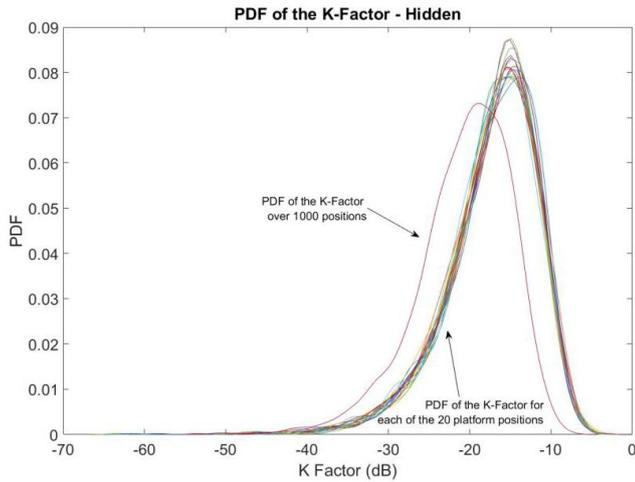
Fig 8. PDFs of K-factors for the hidden antenna combination.
